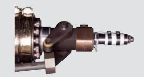
Nozzle shut-off valves allow for recovery during clamp-open, increasing the available overall recovery time. The rotating internal mechanism reduces pressure drop during injection while keeping the moving components at a minimum to ensure reliability during high throughput applications. Nozzle shut-off valve is pneumatically operated.
