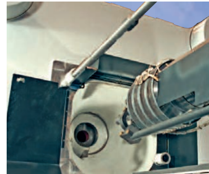
Larger tapered conical hole in the stationary platen provides excellent access to purgings and injection tip for removal.
