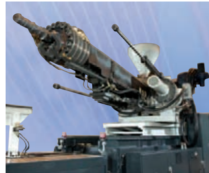
Powered injection unit swivel enables quick and easy access to maintain the screw tip or remove/install feed screws.
