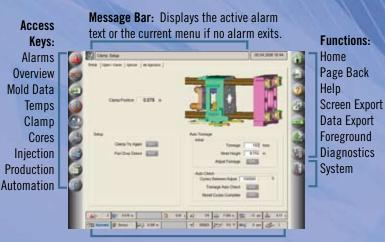
**Status Bar:** The always visible Status Bar provides a quick glance at the current status of critical machine parameters.
