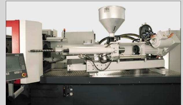
Injection unit swivels for easy maintenance
