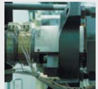
Separate In-Line Packing Pot Assures Straight-Through Material Flow.
