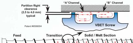
The VBET Solid /Melt Screw keeps the unmelted pellets mixing with fresh melt. VBET's unique channels and undercuts are large enough to allow pellets as well as melt to pass over them. VBET yields significantly higher melting rates because its surface area for unmelted
